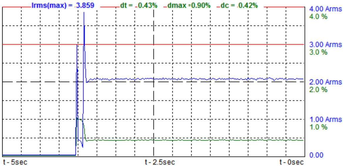
The graph measurement above shows the maximum R.M.S. input current (including inrush current) evaluated over each 10ms half-period between zero-crossings during the worse case switching operation does not exceed 20A.
