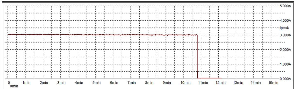
The graph measurement above shows the supply current after initial switch on inrush is within a variation band of 1.5A. The points shown in the graph where the supply current changes was where the product was manually switched off.
